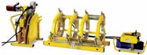
Butt Welding machine for pressure pipes, with basic machine composed by four self-aligning clamps, Electro-hydraulic unit complete of pressure regulator, by-pass and accumulator, ptfe coated heating mirror with electronic thermostat and separate thermometer, electric facing tool with safety micro switch, full set of reducing rings and transport wooden box.
